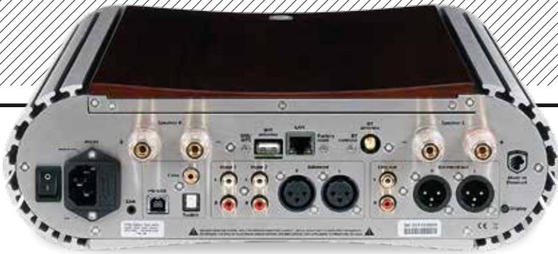
ABOVE: Substantial 4mm speaker outlets, single-ended (RCA) and balanced preamp outs (XLR) are joined by three line inputs (one balanced on XLR). The digital inputs include optical, coaxial, USB-B and LAN plus USB-A (Wi-Fi) and BT antenna sockets
