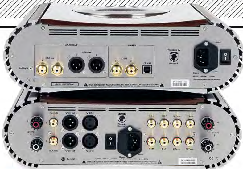
ABOVE: There are balanced inputs to be found on the rear of the AMP-150 to match the balanced outputs on the CDD-1, which also provides high-resolution DAC-only operation with S/PDIF and USB digital inputs
